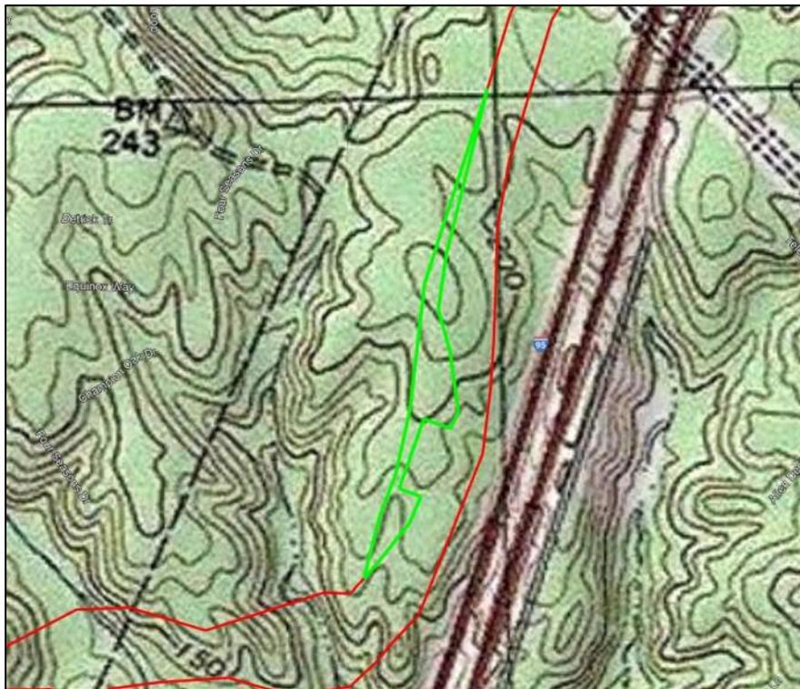
**Figure 1-2: USGS topographic map illustrating the proposed realignment and expanded ROW (green) and the original ROW limits (red). Source: ROW file data provided by Dewberry**
